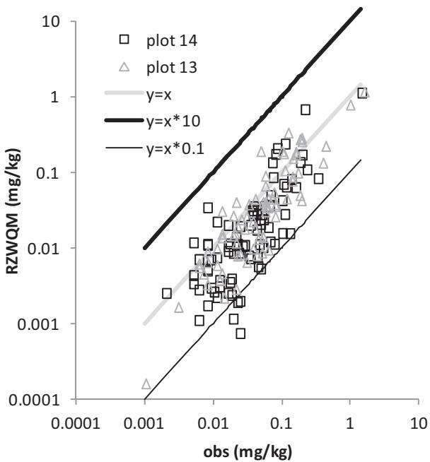
**Fig. 3.** Observed vs. RZWQM simulated atrazine concentration in the soil profile at different depth increments for plots 13 and 14 (1990–1995). Soil concentrations are not presented if observed values were less than 0.001 mg/kg. The two soil concentrations under predicted by more than a factor of 10 are for plot 14 (10–20 cm, May 1995; 0–10 cm, Oct. 1994). Plot 13 is tilled and plot 14 is no-till.
