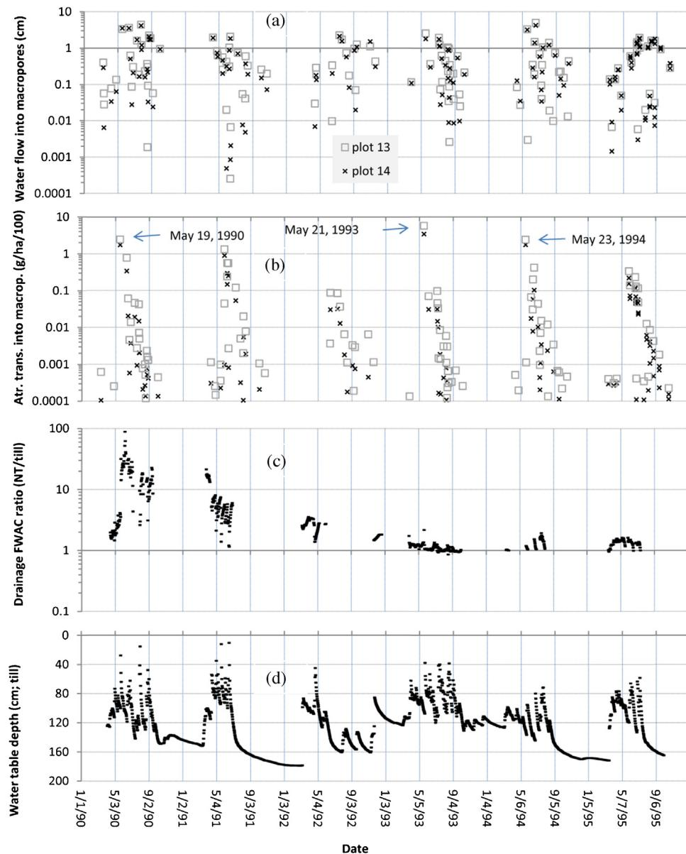
**Fig. 6.** RZWQM daily water table depth, atrazine concentration ratio in drain flow, and macropore flow characteristics. Atrazine was spring applied each year at a rate of 3 kg/ha for both plots 13 and 14. (a) is daily water flow into macropores. (b) is daily atrazine transport into macropores. (c) is daily flow weighted atrazine concentration (FWAC) ratio in drain flow (NT/till). (d) is daily water table depth for plot 13. Plot 13 is till and plot 14 is no-till (NT).
